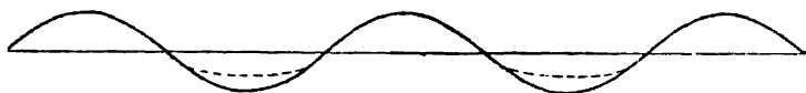
Fig. 60. The response of the ear-drum to a simple sound. The unsymmetrical nature of the human ear results in parts of the simple harmonic curve, which is drawn thick, being replaced by those shewn by broken lines.
